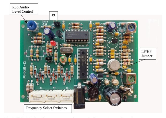
The ACC100 - Version 6 incorporates some changes to facilitate easier assembly and use. The original radio frequency circuitry and the associated parts placement remains exactly the same as in previous versions. There are no changes in the RF characteristics or modulator circuits.
