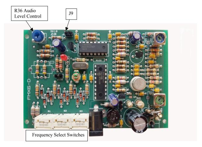
The ACC100D - Version 6 incorporates some changes for easier use. The original radio frequency circuitry and the associated parts placement remains exactly the same as in previous versions. There are no changes in the RF characteristics or modulator circuits.
