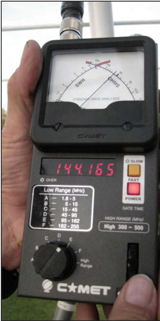
The Comet CAA-500's bright frequency display and precision metering make SWR analysis in the field simple and quick.
