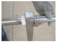
■ Install the brackets over the boom arm in order to have vertical polarization.
