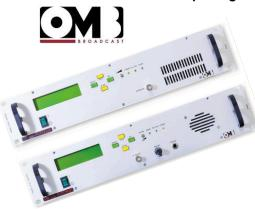
The *OMB* MT/MR < 1 GHz STL system (Studio to Transmitter Link) is used in applications where your main FM transmitter will be in a separate location from the studio. This powerful FCC type accepted 19" rack-mountable STL system can send a clean stereo audio signal to a location UP TO 10 miles away! Frequency is PLL synthesized by a built-in microprocessor. The STL transmitter and receiver pairs are available in 20 MHz bands within the frequency range of 170 MHz to 960 MHz (20 watts).
