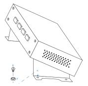
Use the four provided No. 6 screws ("E") and cup washers ("F") as shown in the diagram above to secure the gadget to a plywood surface.
