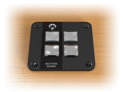
You can use the Button Gizmo with other consoles too. Any console with GPIO logic will easily interface. We include an RJ45 to screw terminal breakout adapter to make it easy to access the contacts.
