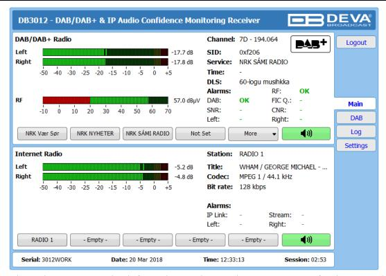
The main screen contains information on the mandatory parameters for the currently selected DAB/DAB+ station and Internet radio. A set of interactive buttons enabling the fast switch between the presets assigned is also available.
