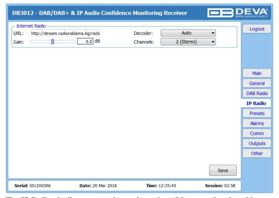
The *IP Radio* tab allows you to change the setting of the currently selected internet stream, or to specify a new one. If a new internet stream is added, the DB3012 will automatically switch to it upon pressing the [Save] button.
