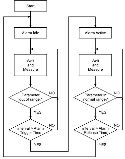
Block Diagram of Alarm Automata
