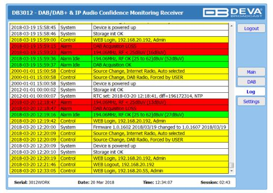
Here are listed all the Device System Events. The local measurements and logs are saved in the internal device memory. All log files can be downloaded via the built-in FTP server. For information on how the connection between the DB3012 and an FTP Client should be configured, please refer to "Download files via FTP" on page 57.
