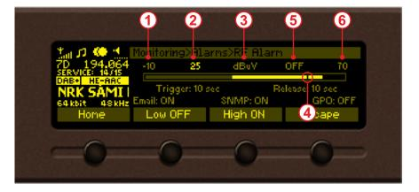
The bar graph indicates the signal range of the alarm. The highlighted area represents the permitted signal value range. If current signal value (pos. 4) is in this range, no alarm event will be generated. Basic elements of the alarm editor dialog:
