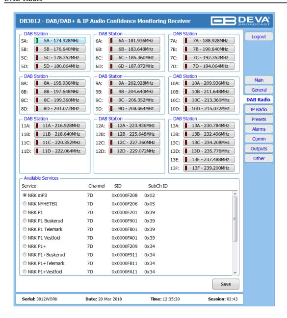
The Tuner Section gives control over Tuner settings, allowing you to select a DAB channel and service. All available services will be listed below once the list is collected from the multiplex data.
