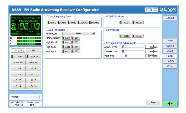
The Tuner Section gives full control over Tuner settings.
