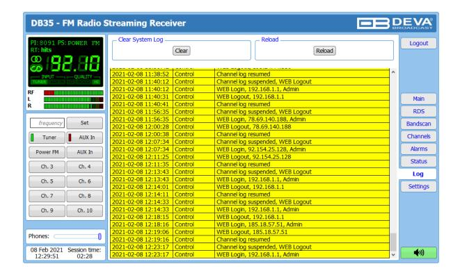
Here are listed all the Device System Events. The local measurements and logs are saved in the internal device memory. All log files can be downloaded via the built-in FTP server. For information on how the connection between the DB35 and an FTP Client should be configured, please refer to "Download files via FTP" on page 37.
