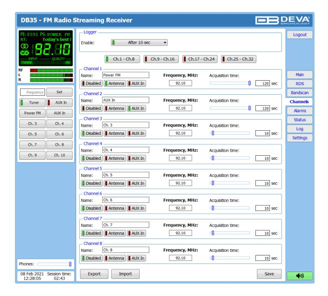
The DB35 can monitor up to 32 FM Stations at regular intervals and send warning and alarm notifications via E-mail and SNMP. Every Channel consists of a group of settings (explained in details below), which are used when monitoring.
