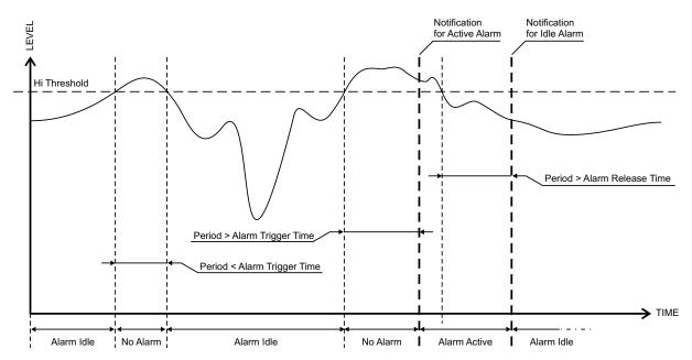
If the RDS Group has not been received within the Alarm Trigger Time, the state would be changed into Active. If the Active state and the Release Time have elapsed and the RDS Group is received, the state is changed to Idle. Should the RDS Group is received before the Release Time is elapsed, the state would remain Active.
