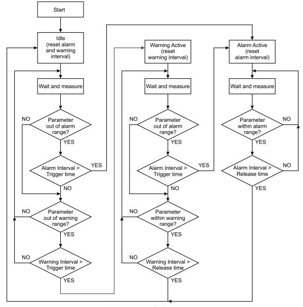
Block Diagram of Alarm Automata
