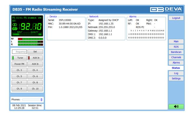
The status tab shows the alarm status of each parameter of the preset frequencies, along with the basic device and network status (IP address, MAC, etc.).
