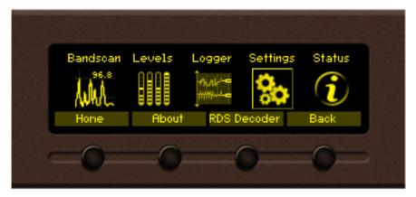
The Settings menu is organized into a hierarchical tree menu and all similar parameters are grouped into sections (branches). The structure of the menu is shown below.
