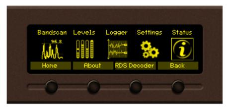
Press the "OK" Button to enter the "Status Section". Via the Front panel navigational menu press the "DOWN" button.
