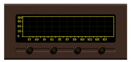
To ensure better reading of the data plot, the Header area and the Soft Buttons labels will be hidden automatically a short time after the soft button is released. Pressing a button will display the function labels again.
