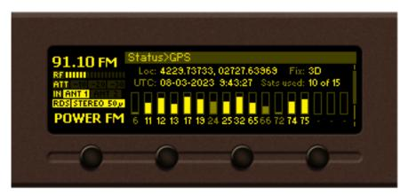
Loc: The current location of the device - Longitude and Latitude in degrees.
